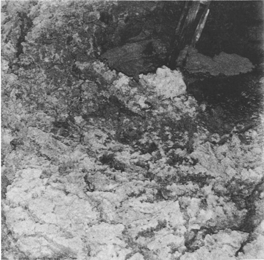
Figure 2. Salt cake in underground storage tank
